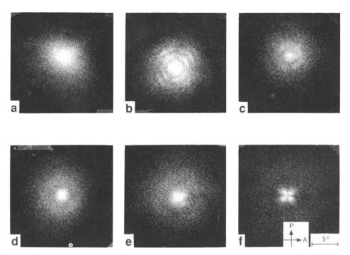
**Figure 3** H<sub>v</sub> light scattering patterns of PCL/SAN blends with different compositions crystallized at 40°C for 3 days from melting 80°C for 7 h and then cooled slowly to 40°C at a rate of 0.16°C min<sup>-1</sup>. (a)–(f) as in *Figure 1*
