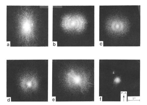
Figure 4  $V_v$  light scattering patterns of PCL/SAN blends with different compositions crystallized at 40°C for 3 days from melting 80°C for 7 h and then cooled slowly to 40°C at a rate of 0.16°C min<sup>-1</sup>. (a)–(f) as in Figure 1
