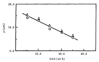
Figure 2 Periodicity of helicoidal crystal orientation within spherulites of blends as a function of weight fraction of SAN: ( $\Delta$ ) light scattering; ( $\bigcirc$ ) optical microscopy
