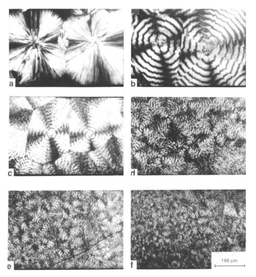
Figure 1 Polarized light micrographs of PCL/SAN blends with different compositions crystallized at 40°C for 3 days from melting at 80°C for 7 h and then cooled slowly to 40°C at a rate of  $0.16^{\circ}$ C min<sup>-1</sup>: (a) 100% PCL; (b) 90/10 PCL/SAN; (c) 80/20 PCL/SAN; (d) 70/30 PCL/SAN; (e) 60/40 PCL/SAN; (f) 50/50 PCL/SAN
